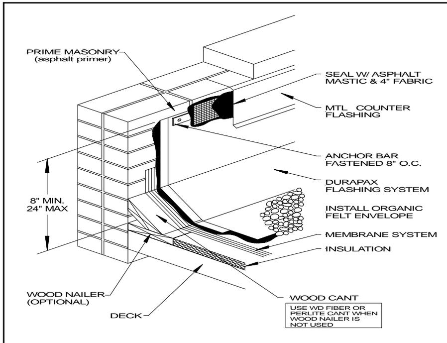
*pax FL-0030 SBS Flashing in steep asphalt, the wall and the back of each ply are to be coated and each sheet pressed into place to assure proper adhesion. All flashing side laps must utilize the selvage edge as the lower ply of the lap. A small amount of bleed out is desired at the laps edge.*
